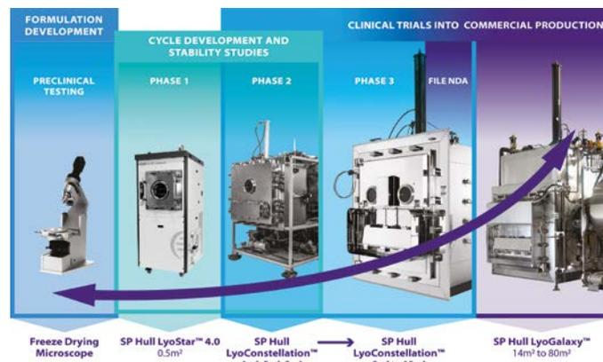
**Figure 1:** Lyophilization Scale-up From Formulation to Full Commercialization
