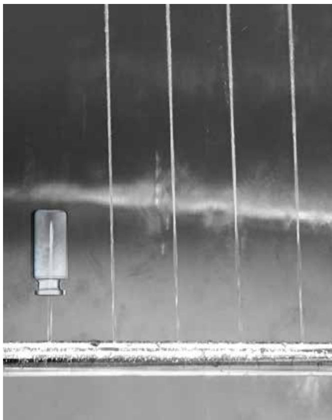
**Figure 3: High Pressure Washing Jet Manifold for Vial Washing Without Needles**
