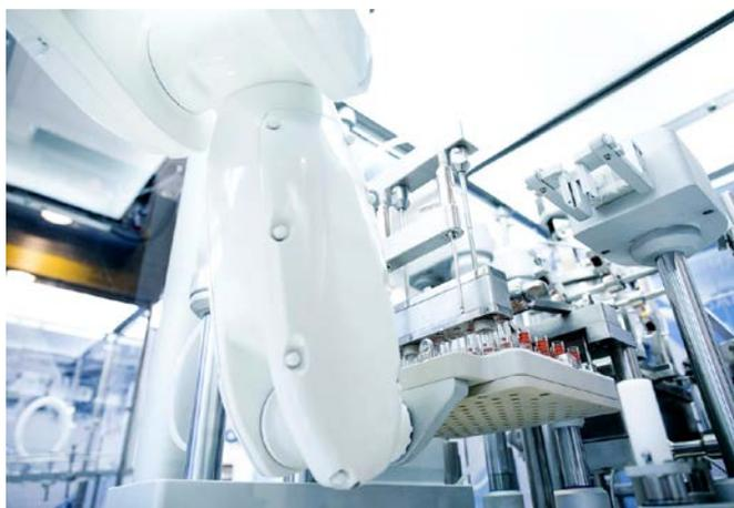
*Robot arm for cartridge filling*
