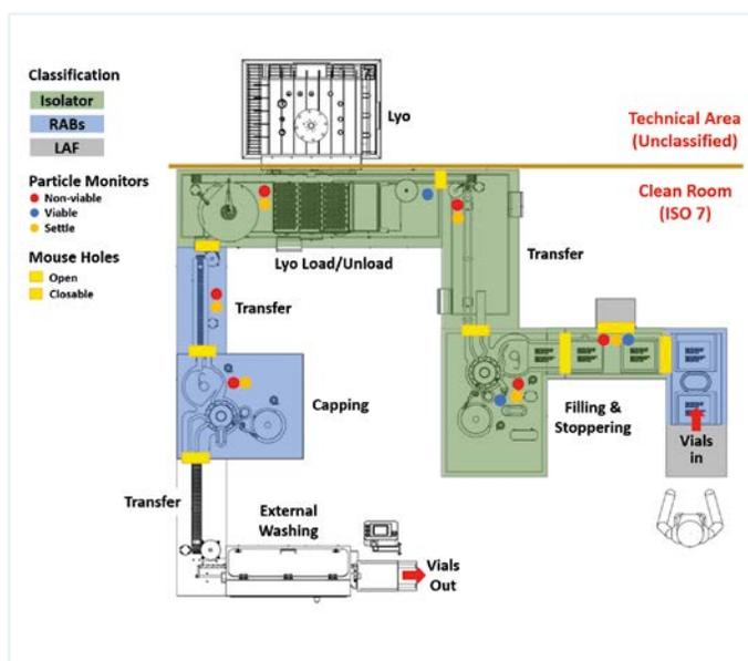
**Figure 6:** Aseptic Fill-Finish Line Showing Zoning and Locations of Particle Monitors
